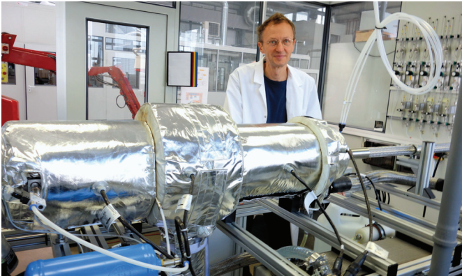
Dipl.-Ing. Achim Hugo testet abreinigbare Filter am VDI-3926-Prüfstand
