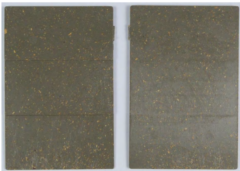
Fig. 6: Stepped plates from rPP/vPP/flax/MAPP compound, front (left) and back (right)
