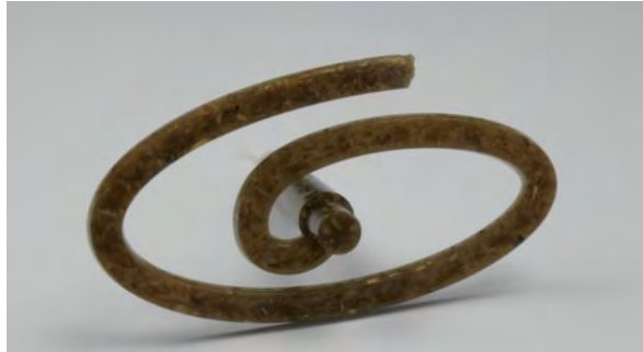
Fig. 3: Spiral flow from PLA/flax compound before and after optimizing process parameters
