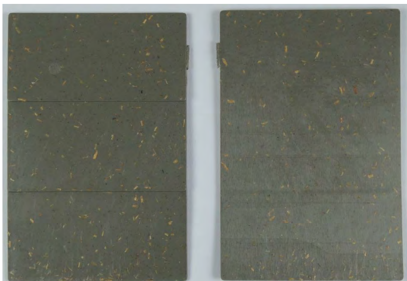
Fig. 5: Stepped plates from rPP/flax compound, front (left) and back (right), color of rPP is light grey
