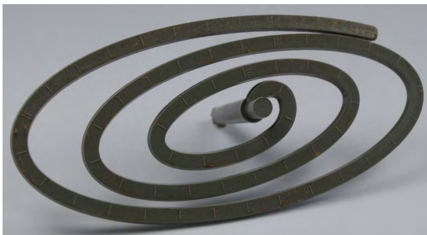
Fig. 9: Spiral flow from rPP/flax compound
