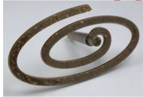
Fig. 3: Spiral flow from PLA/flax compound before and after optimizing process parameters
